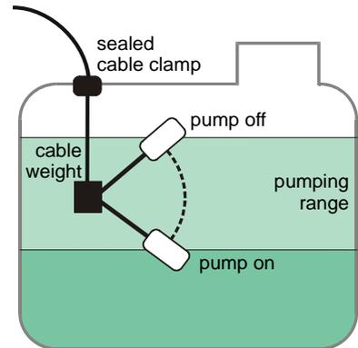
**Grounding shielded float switch cable** If you use shielded cable, connect the shield to ground AT THE CONTROLLER ONLY. DO NOT ground the shield at the float switch. This will reduce surges induced by nearby lightning.
