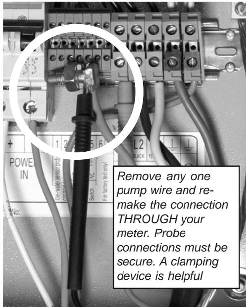
Remove any one pump wire and re-make the connection **THROUGH** your meter. Probe connections must be secure. A clamping device is helpful
