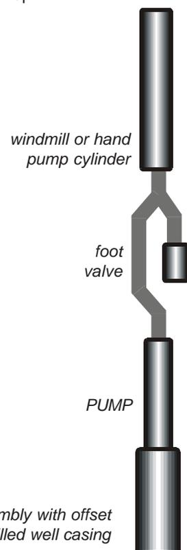
*Bypass foot valve assembly with offset elbows to fit a drilled well casing*
