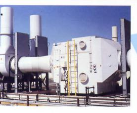
his version of the horizontal packed scrubber system incorporates standard ANSI pumps, which recirculate the scrubbing liquor. Pump construction is based on specific chemistry; standard pump heads are available in FRP, polypropylene and stainless steel. Other materials are available for unique applications.
